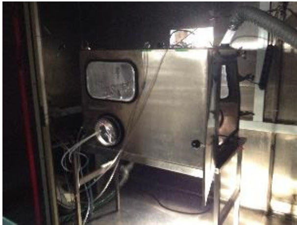
Figure 3. The glove box of 0.38 m 3 used to condition vented gases and aerosols.
