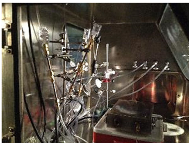
Figure 4. Inside the glove box with all sampling equipment setup and the battery box on the heater ready to receive thermal load until ventilation.
