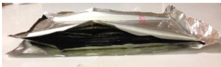
Figure 5. Ruptured pouch cell of LFP type. NMC type is similar.
